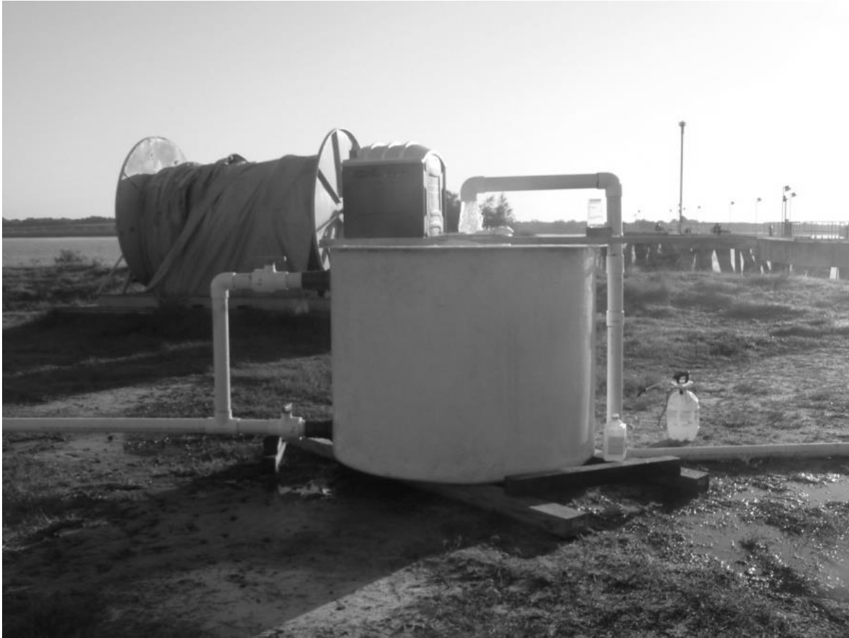
Figure 3. Side view of the sampling apparatus showing water flowing into the center of the tank.
