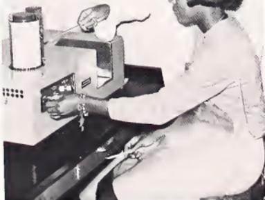
Dr. Raut and research student, Jamie Singleton, test a solution in the new Infrared Spectrophotometer.
